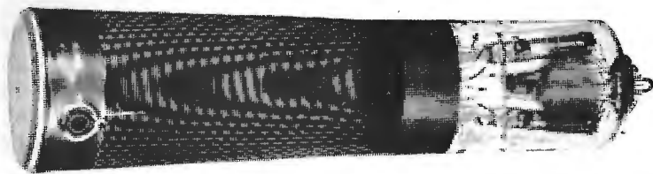
Above: Double-beam oscilloscope tube, Type E10-10GH ("La Radio-technique").
